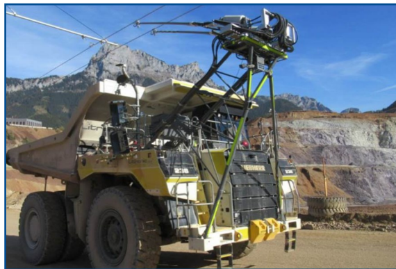
▲ This Trolley Assist Haul Truck system is one example of technologies used in the mining industry that will facilitate the transition to autonomous battery electric vehicles.
